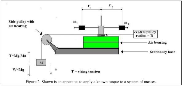
The vertical acceleration, a, is obtained using the time, t, it takes for the mass (M) to fall from the starting elevation,  $y = \frac{1}{2}at^2$  ( $a = 2y/t^2$ ). The angular acceleration,  $\alpha$ , is obtained from the linear acceleration using  $\alpha = a/R$ .
