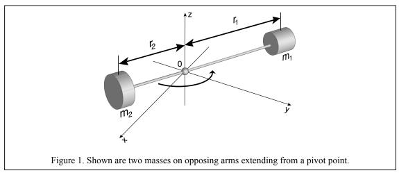
about a pivot point, with point masses  $m_1$  and  $m_2$ , located at distances  $r_1$  and  $r_2$  from the pivot, as shown in Figure 1, the Moment of Inertia is given by,  $I = m_1 r_1^2 + m_2 r_2^2$ . When the arms are not mass-less and/or the masses are not point masses, the moment of inertia will include a constant,  $I_0$ , which accounts for the distribution of mass in each of these components, so that the Moment of Inertia becomes,  $I = m_1 r_1^2 + m_2 r_2^2 + I_0$ . The equation is
