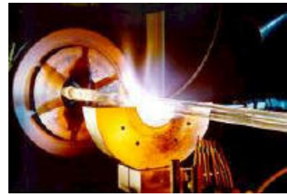
Photo courtesy Fibercore Ltd. Lathe used in preparing the preform blank
