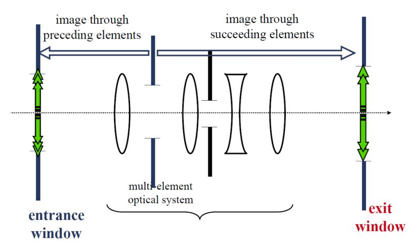
The image of the field stop as seen through all the optics before the field stop is called the **entrance window**. The image as seen through all the optics after the field stop is called the **exit window**.
