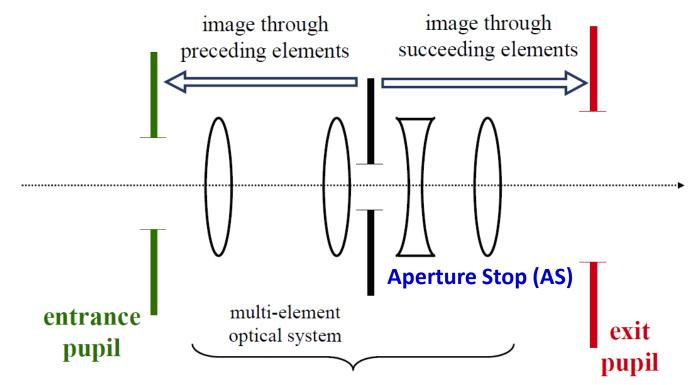
The **aperture stop** (AS) is defined to be the stop or lens ring, which physically limits the solid angle of rays passing through the system from an **on-axis** object point. The aperture stop limits the brightness of an image.
