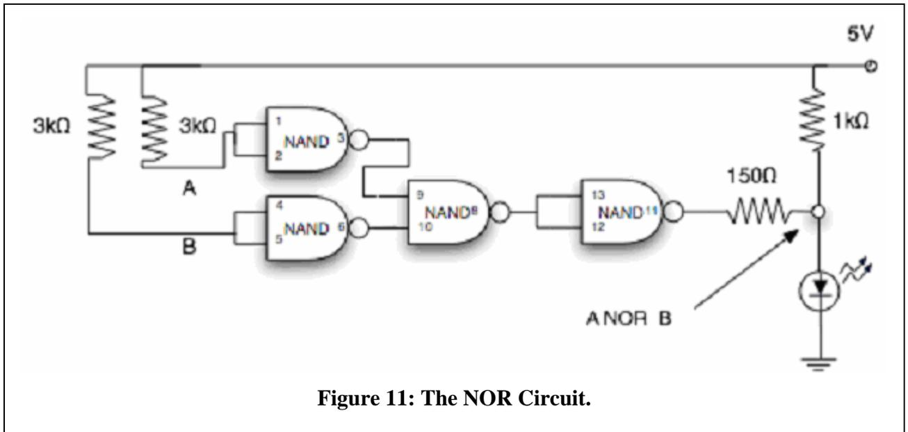
**Figure 11: The NOR Circuit.**
