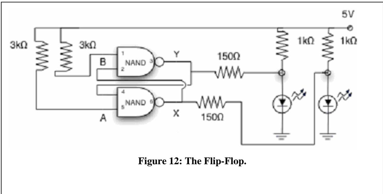
**Figure 12: The Flip-Flop.**
