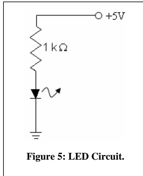
**Figure 5: LED Circuit.**
