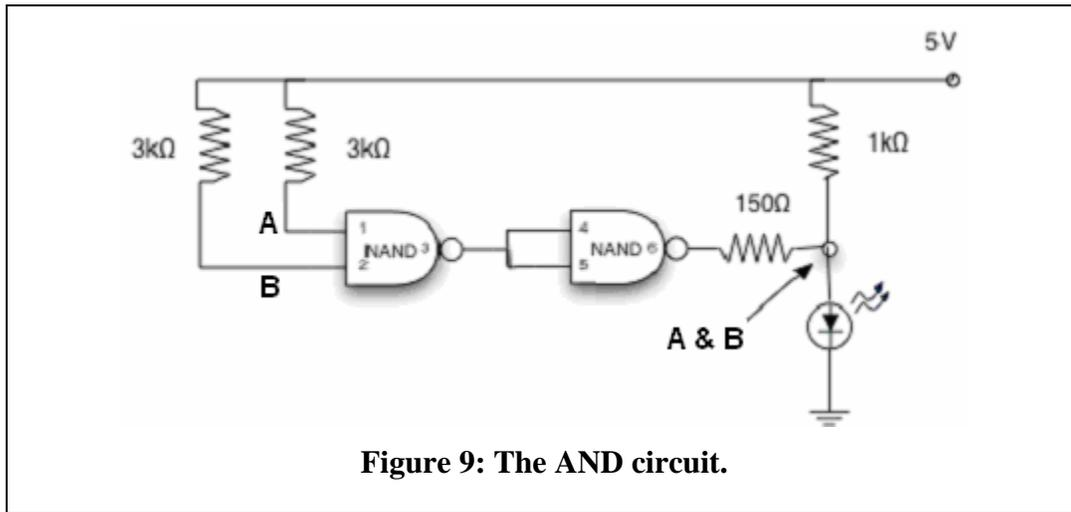
Figure 9: The AND circuit.
