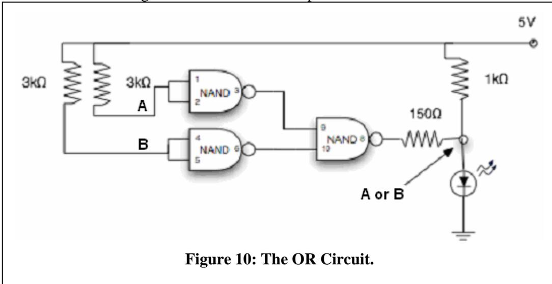
**Figure 10: The OR Circuit.**
