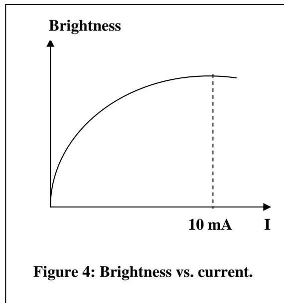
**Figure 4: Brightness vs. current.**
