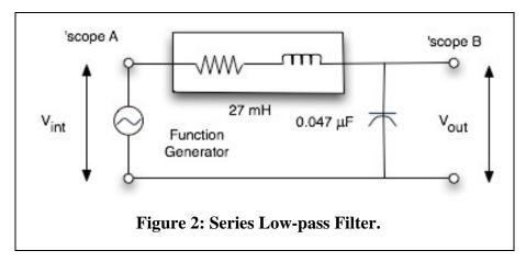
of the inductor plus any resistance contributed by the Function Generator. Normally the Function Generator has an output impedance of 50  $\Omega$ . Verify that this is the case by measuring the resistance of the function generator output with the generator turned on but the output voltage set to 20 mV (the lowest setting). Measure the resistance of the inductor, add the value contributed by the Function Generator and use this sum in your calculations below.
