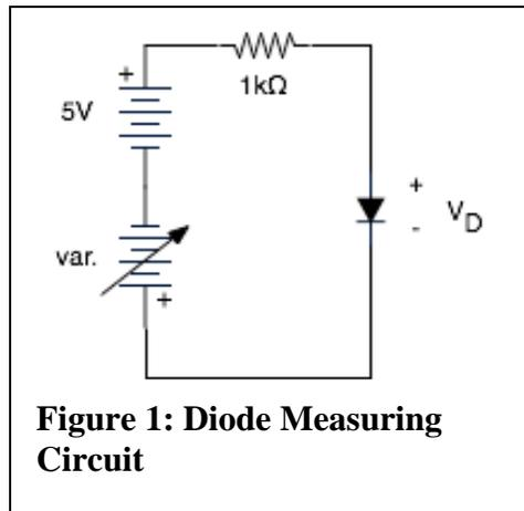
**Figure 1: Diode Measuring Circuit**
