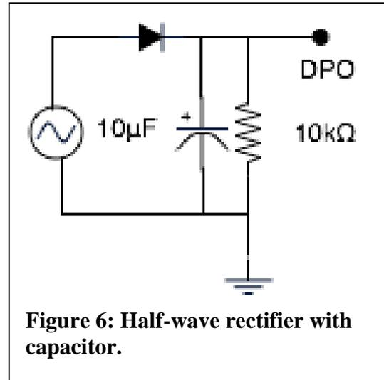
The capacitor is electrolytic. You must obey the polarity markings when you connect this capacitor in the circuit.
