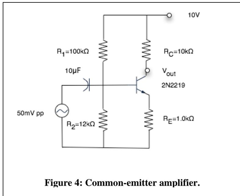
**Figure 4: Common-emitter amplifier.**
