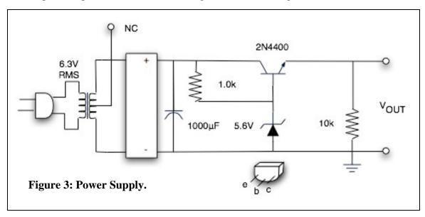
The rectangular box refers to the full-wave rectifier WL02F. and "NC" means no connections to the center tap on the transformer The output should be about 5 volts.
