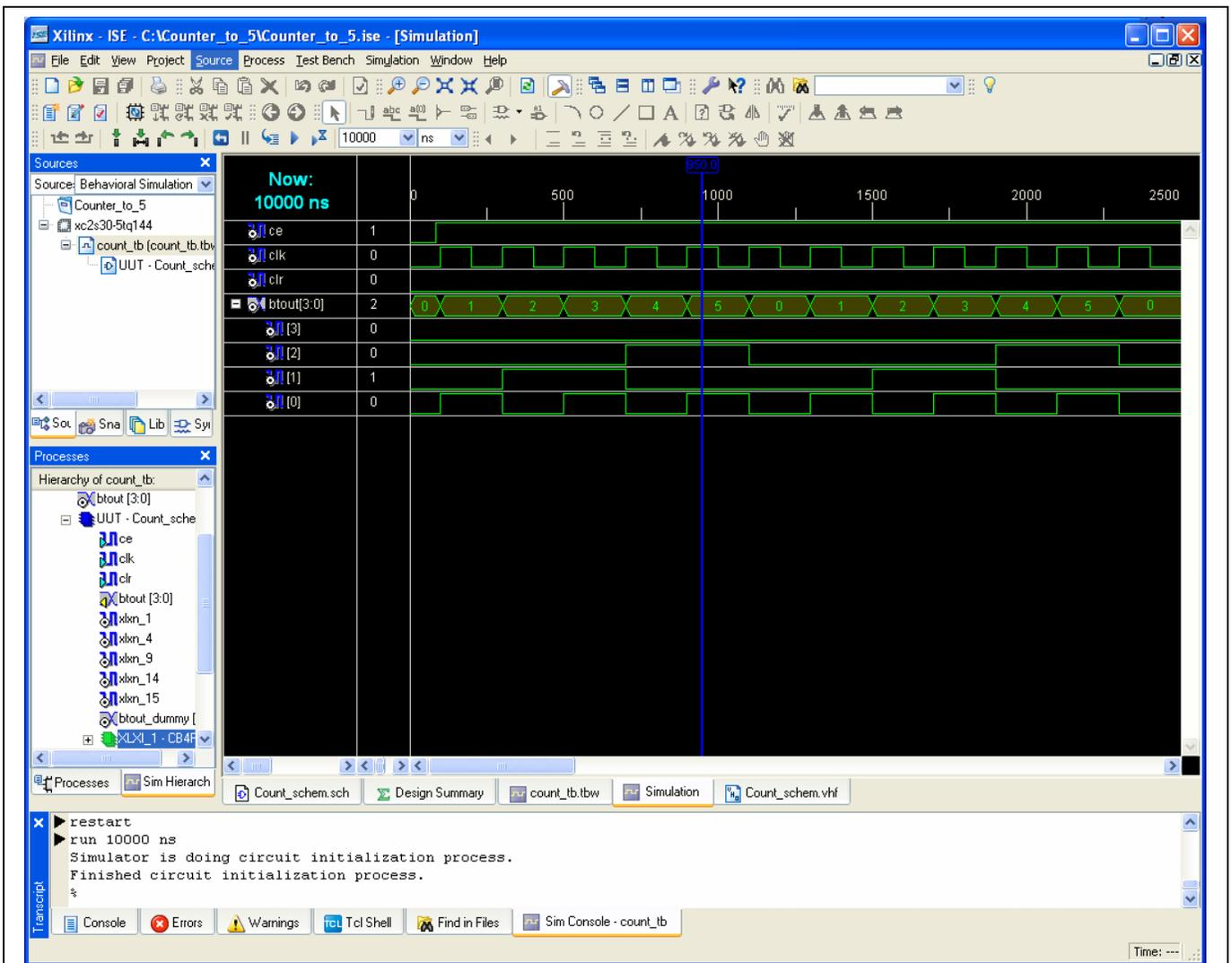
Figure 11: Testbench Waveforms for 0 to 5 Counter
