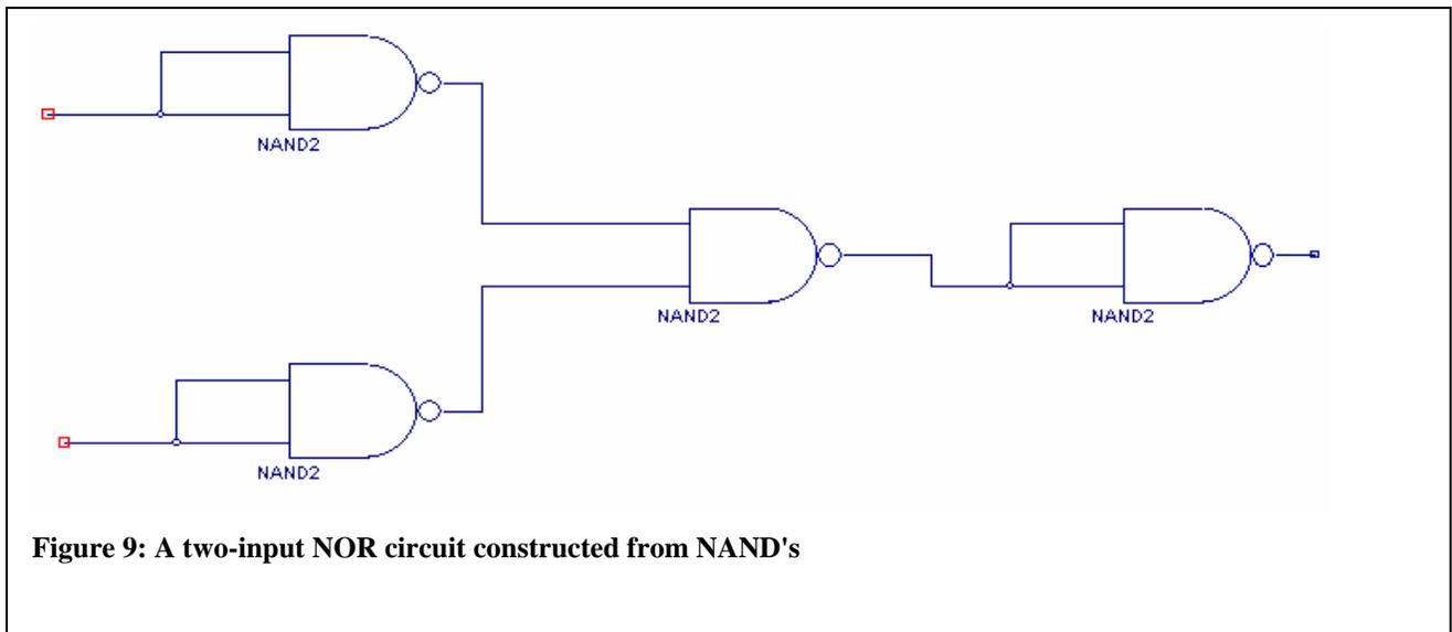
in Figure 9 which creates a NOR gate from 4 NAND's. Finish the circuit by adding input and output (I/O) buffers and giving appropriate labels to the I/O lines. You can once again use BTN1 and BTN2 for inputs and LD1 for the output. Verify that the truth table for a two-input NOR gate is satisfied.
