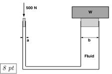
Consider the hydraulic system shown above. A force of 500 N is applied as shown on the piston to the left which has a diameter of a=2 cm. The piston on the right has a diameter b=7 cm. What weight W (in N) can be lifted with this force? (Ignore friction and the weights of the piston)
