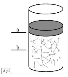
▷ A massive piston traps a fixed amount of helium gas as shown. After being brought to point (a) the system equilibrates at room temperature. Weight is then added to the piston adiabatically compressing the gas to half of its original volume (b). The internal energy of the gas at "b" is the internal energy of the gas at "a".
