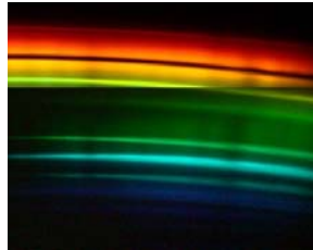
e). A high pressure sodium lamp (modern street light). Notice the strong Sodium absorption (black line) in the Yellow).
