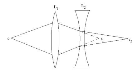
C. Calculate the index of refraction (including uncertainty) for the glass of your lens using the lensmaker's equation. Compare this with the value found in Part I.
