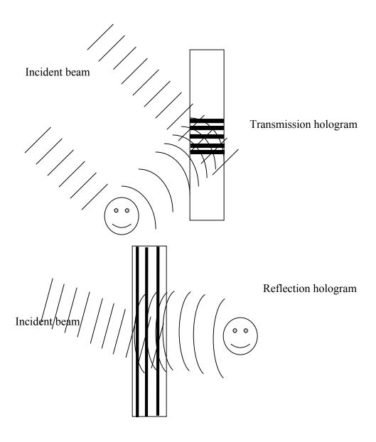
Reflection of light off one of these planes follows the Bragg equation  $\lambda = 2d \sin \theta$  where d is the spacing between planes,  $\lambda$  is the wavelength and  $\theta$  is the angle of incident light for viewing. The emulsion on the plates is much thicker (~7 microns) than the wavelength so multiple planes of fringes are created in the reflection hologram.
