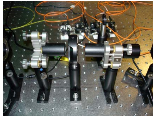
Fig. 3. The BDP's. The large black "knob" on the mount on the right is a stepper motor. It allows the computer to tilt the mount to adjust the phase,
