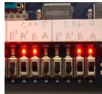
Figure 5: How the switches determine which coincidence is counted. Here, Counter 4 will count AB coincidences, and Counter 5 will count A'B coincidences.
