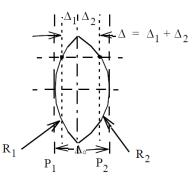
In propagating from plane  $P_1$  to  $P_2$ , the light travels a distance  $\Delta = \Delta_1 + \Delta_2$  in the glass and a distance  $\Delta_{\circ} - \Delta$  in air, where  $\Delta_{\circ}$  is the thickness at the thickest part of the lens. The phase delay depends on (x, y):
