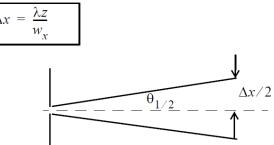
For a circular aperture with radius w:  $t_A = circ(\frac{q}{w})$   $q^2 = \xi^2 + \eta^2$  radial coordinates
