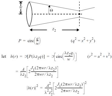
The spot diameter is  $d = 1.22 \frac{\lambda f}{w} = 1.22 \frac{\lambda}{\theta}$ The resolution of the lens as defined by the "Rayleigh" criterion is  $d/2 = 0.61\lambda/\theta$ . For a small angle  $\theta$ ,  $d/2 = 0.61\lambda/\sin\theta = 0.61 \frac{\lambda}{NA}$ .
