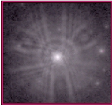
Figure 1.15 Spherical aberration of a plano-convex lens
