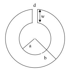
$\vec{\nabla} \times \vec{H} = \frac{4\pi}{c} \vec{j}$  and the boundary condition on  $B_{\perp}$  at the pole pieces.
