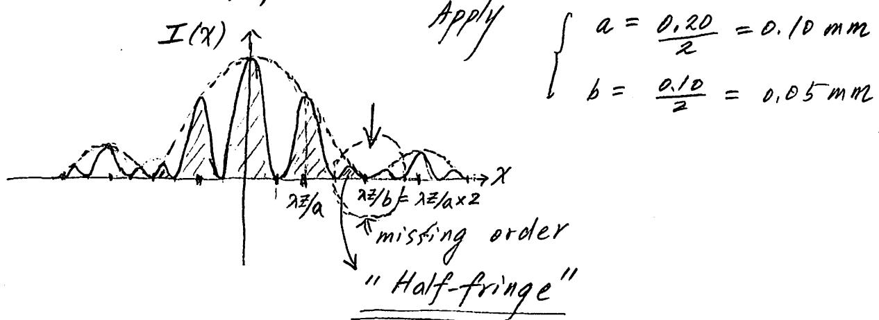
A sketch of the diffraction pattern is shown for  $a/b = 2$ . The missing order occurs at  $\lambda z/b = 2 \cdot \frac{\lambda z}{a}$ , and the fringe next to it is counted as "half".
