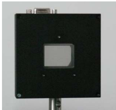
Figure 9: The upright LC2002-light modulator with the connections on top
