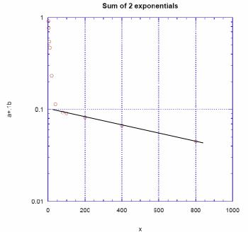
A good way to deal with this situation is to fit data for the flatter attenuation curve first (ie at larger x), since the other radiation source will have died out and not contaminate the second, "slower" attenuation curve very much. In the example curve above, the last 4-5 points lie on a good straight line, even though the data is actually a sum of two exponentials,
