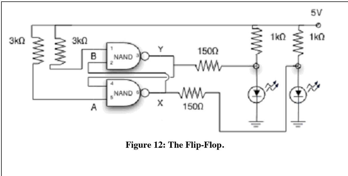
**Figure 12: The Flip-Flop.**
