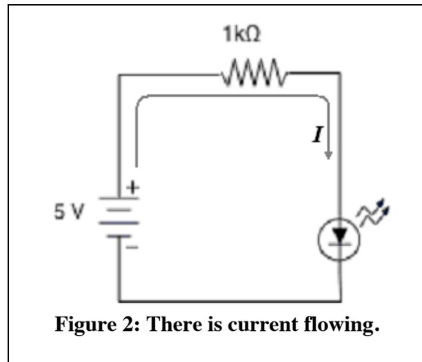
In Figure 1 the diode is biased in the backward direction or “reverse biased” and there is no current flowing through it whereas in Figure 2 the diode is “forward biased” and there is current flowing.
