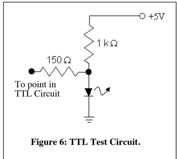
(mA) is directly equal to the voltage in volts). Observe the increasing brightness as a function of current as you increase the supply voltage. You should find that a current between 5 and 10 mA gives a normal glow.
