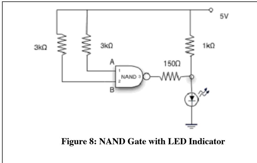
The 3k resistors pull the two inputs to a high state. According to the NAND truth table this is the only input configuration where the output is low and the LED is off. Points A and B may be grounded by means of a wire going to ground to bring them to a low state. In this way you can create a zero on the input.
