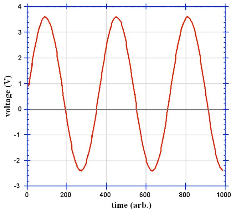
**Figure 2: A 3 V sine wave (6 V peak-to-peak) with 0.6 V DC offset.**
