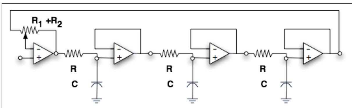
\*Show that the transfer function for the low-pass resonant filter, shown in Figure 2, is given by:
