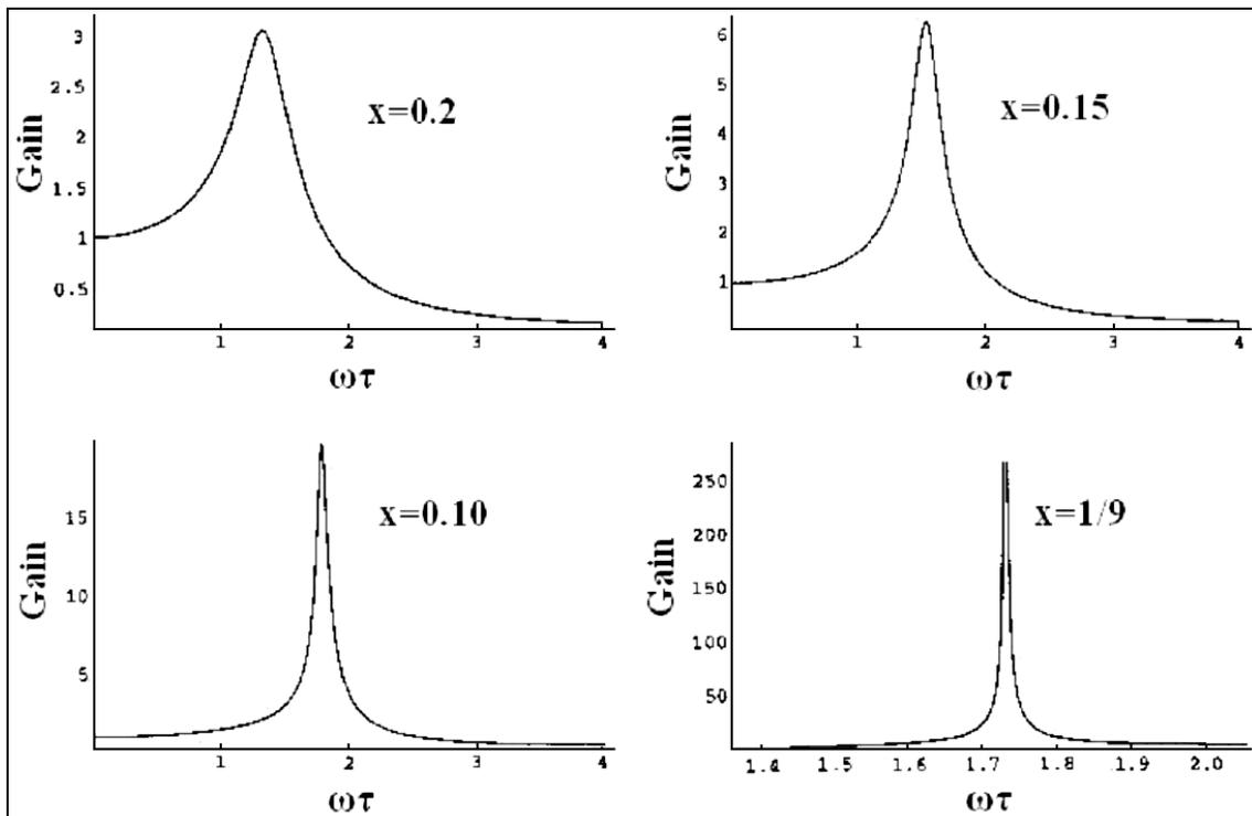
Figure 3: Gain of the low-pass resonant filter for different resistance ratios.
