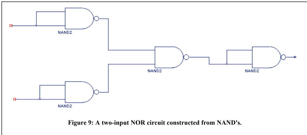
in Figure 9 which creates a NOR gate from 4 NAND's. Finish the circuit by adding input and output (I/O) buffers and giving appropriate labels to the I/O lines. You can once again use BTN1 and BTN2 for inputs and LD1 for the output. Verify that the truth table for a two-input NOR gate is satisfied.
