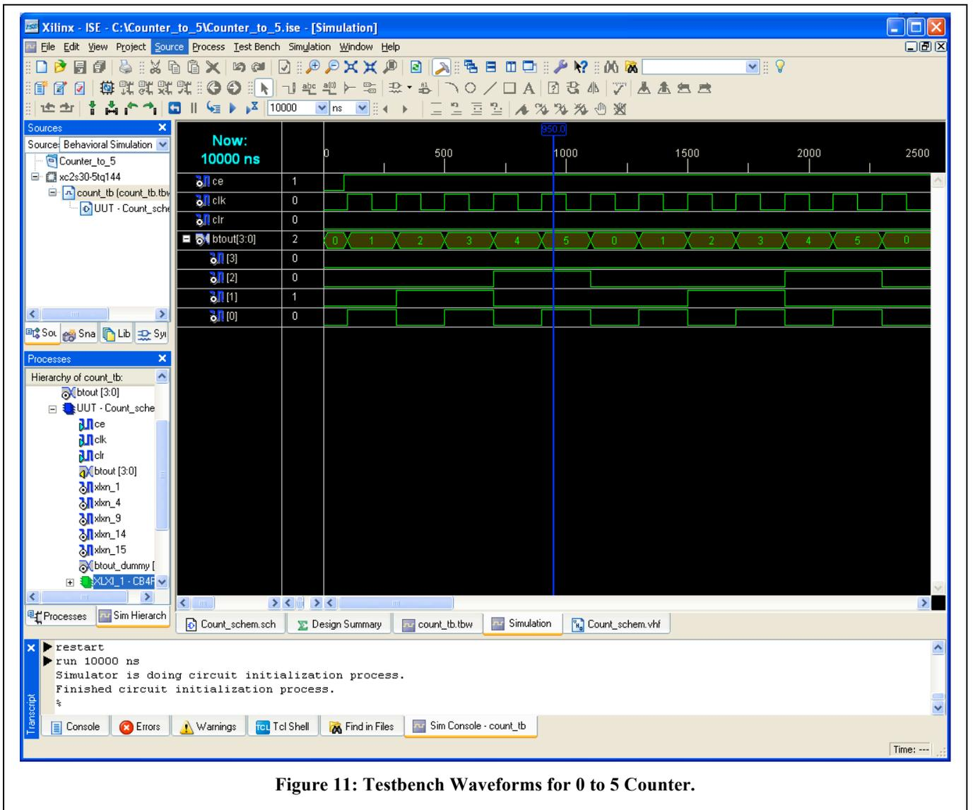
Figure 11: Testbench Waveforms for 0 to 5 Counter.
