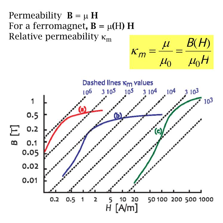
(a) Supermalloy; (b) Mumetal; (c) Iron Ni(79%)Mo(5%)Fe(16%) Ni(77)Fe(15)Cu(4)Mo(4) Fe
