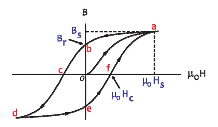
$B_s$  = saturation field (all domains aligned)  $B_r$  = remanent field (permanent magnet)  $H_c$  = coercive force (static field required to demagnetize the sample)
