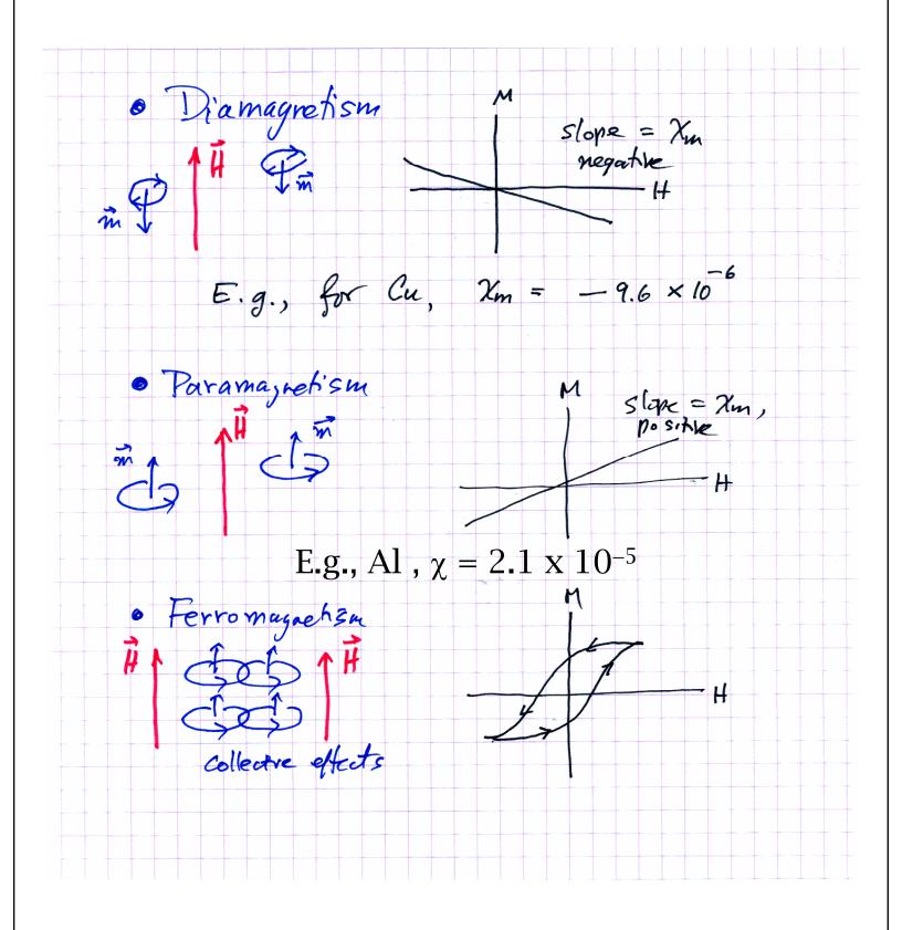
9.5/2 Magnetic Domains Consider a non-magnetized bar of irm. Macroscopically, M(x) = 0. But in small domains, all the atomic dipoles are aligned by the "exchange interaction," a quantum effect.
