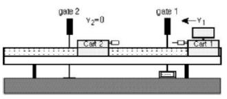
Figure 1: Initial state of the carts before inelastic collision (fin on cart 2 can be removed). **Warning**: *your carts should be balanced, unlike the ones in this figure!*
