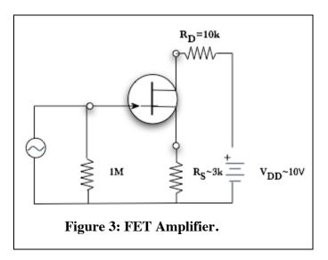
The circuit above is an AC amplifier. The output signal at the drain will be larger than the input signal on the gate.
