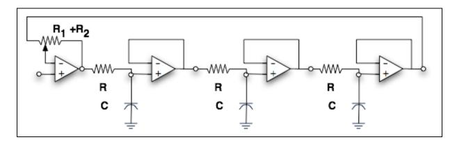
Figure 2: Low-pass resonant filter.
