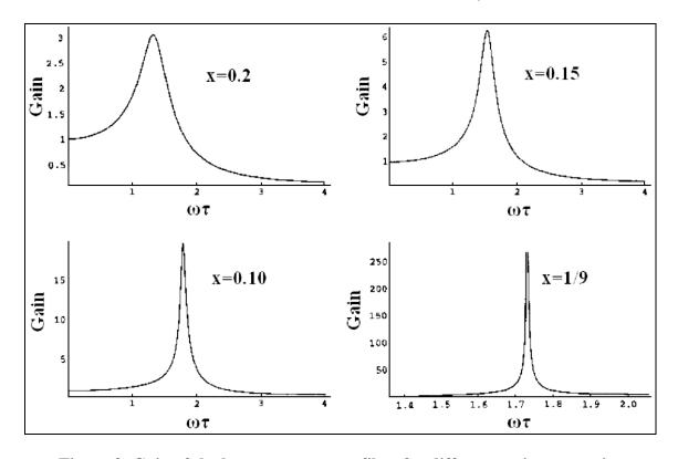
Figure 3: Gain of the low-pass resonant filter for different resistance ratios.
