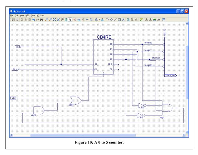
with their names specified by using the netname tool. In our case these names are btout(0) to btout(3). You may need to use the "Rotate" command located in the "Edit" menu to orient the bus tabs properly.
