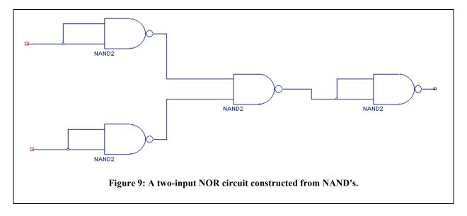
in Figure 9 which creates a NOR gate from 4 NAND's. Finish the circuit by adding input and output (I/O) buffers and giving appropriate labels to the I/O lines. You can once again use BTN1 and BTN2 for inputs and LD1 for the output. Verify that the truth table for a two-input NOR gate is satisfied.
