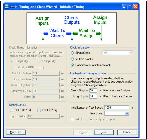
Figure 6: Timing choices for ISE simulator.
