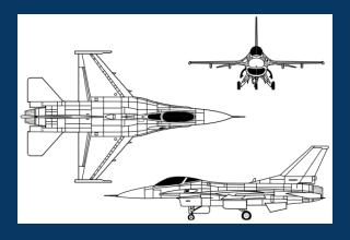
F-16 Mass (loaded, takeoff) = 15,000 kg Max speed = Mach 2 = 2410 km/h = 670 m/s
