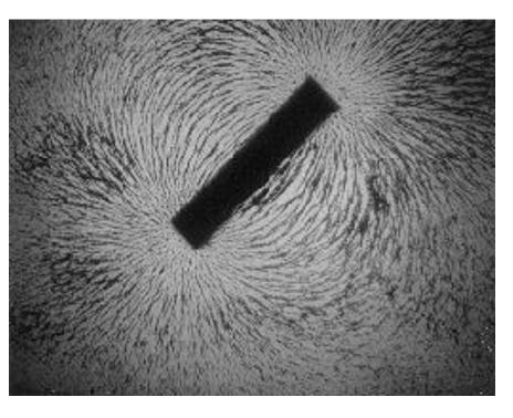
Iron filings trace out the magnetic field lines around a bar magnet.
