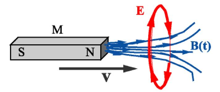
Lenz's law: If a conductor is present, the induced electric field opposes the change of the magnetic field.
