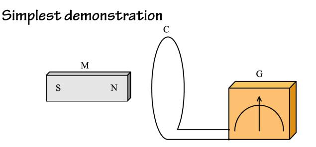
When M moves, a current flows around C and produces a deflection of the galvanometer needle.
