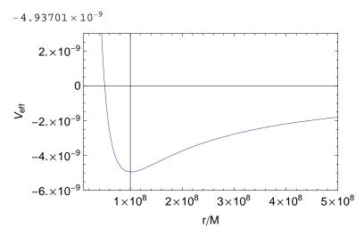
Caption:  $V_{\text{eff}}(r)$  for Earth's orbit. The energy 0.8  $\mathcal{E}$  is shown to make it visible. The dimensionless angular momentum is 10063.6. Q: For what energy or range of energies is the orbit elliptical? Parabolic? Hyperbolic?
