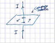
[2.] Electric currents exert forces on each other. (Ampere, 1820) This is an example of magnetism.
