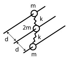
4. [5 pts] Consider three identical pendula suspended from a slightly yielding support. Because the support is not rigid, a coupling occurs between the pendula, making the potential energy approximately equal to:
