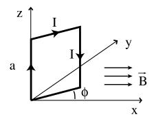
$$L(\phi, \dot{\phi}, q, \dot{q}) = \frac{1}{2} J \dot{\phi}^2 + \frac{1}{2} \mathcal{L} \dot{q}^2 - \dot{q} a^2 B \sin \phi.$$
