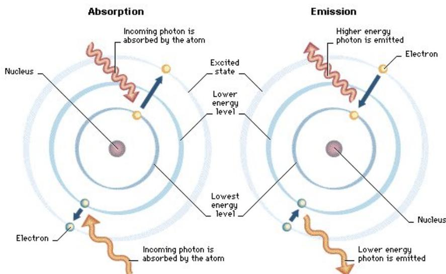
Figure 10.3: Model of an atom showing absorption and emission of photons.
