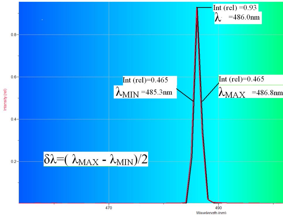
Figure 10.11: Example of how to label the graphs of emission spectra to find the HWHM. This graph shows the zoomed in x-axis used for the laser but your other sources should show the entire visible wavelength range.
