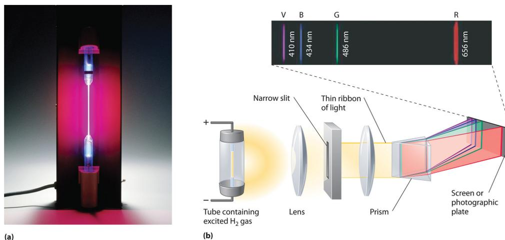
Figure 10.5: (a) A discharge tube containing hydrogen gas. (b) The experimental setup used to obtain an emission spectrum for hydrogen with the wavelengths of the 4 visible emission lines noted.
