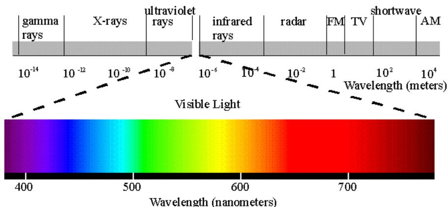
Figure 10.1: The electromagnetic spectrum with the visible light region blown up.
