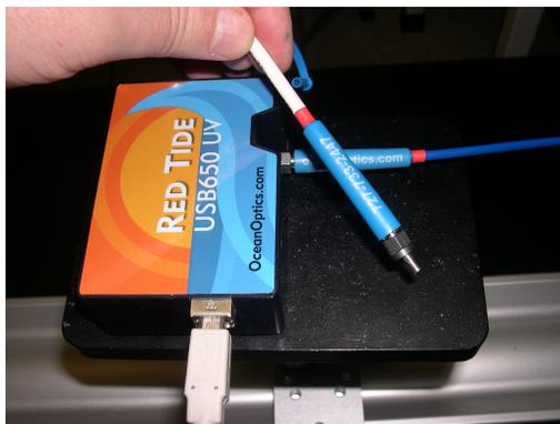
Figure 10.8: The digital spectrometer with a white USB cable and blue optical fiber plugged in.
