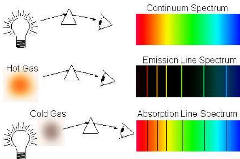
Figure 10.2: Examples of a continuous, an emission and an absorption spectrum with diagrams illustrating how the spectra were obtained.
