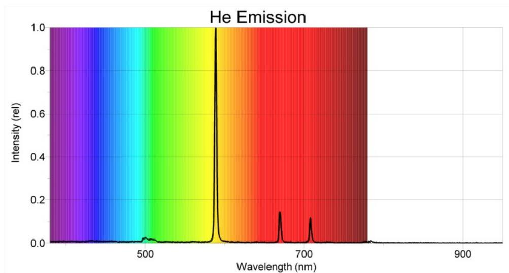
Figure 10.10: An example of an Helium emission spectrum, similar to what you will see on the computer screen.
