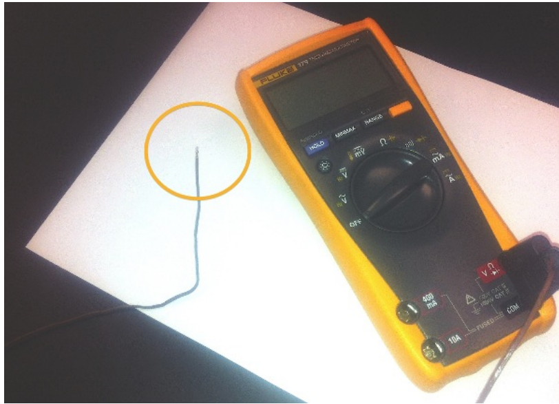
Figure 3.2: A thermocouple is a device that will respond to tiny changes in temperature (circled). It's attached to the multimeter.
