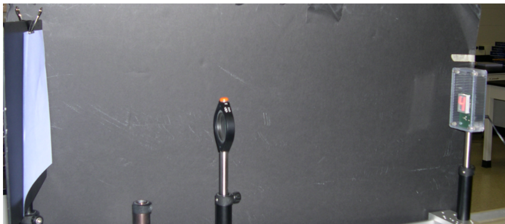
Figure 8.6: Optics bench with an object, a converging lens and a screen.
