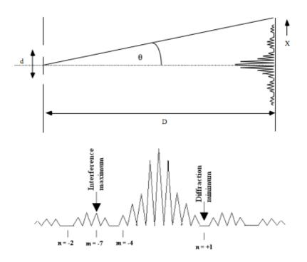
Figure 9.9: Geometry and intensity distribution for double-slit diffraction and interference. Arrows point to the m = -7 interference maximum and the n = +1 diffraction minimum. Note that the m = -5 interference maximum is not seen here as it coincides with the n = -1 diffraction minimum.
