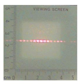
Figure 9.6: Diffraction and interference pattern produced by laser light passing through a double-slit.
