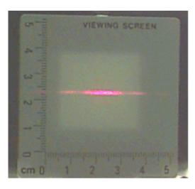
Figure 9.2: Diffraction pattern produced by laser light passing through a single slit.
