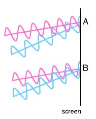
Figure 9.1: Two waves (one pink and one blue) impinging on a screen from a slit arrangement (unseen from the left). The top picture shows 2 waves out of phase with each other and combining destructively at point A. The bottom pictures shows 2 waves in phase with each other and combining constructively at point B.
