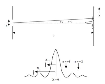
Figure 9.4: Geometry and intensity distribution in single-slit diffraction. The diagrams are labeled with the variables used in the diffraction equation.
