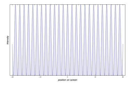
Figure 9.7: Intensity of light from only the two slits interfering with each other, not from the light from different edges of the same slit.
