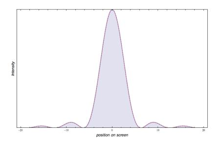
Figure 9.3: A plot of the intensity of light from diffraction through a singleslit as a function of position on the screen.
