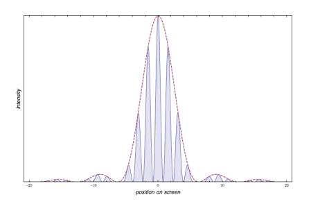
Figure 9.8: Intensity of light from a double-slit showing both the interference effect from 2 slits and the diffraction effect from within a slit. The diffraction pattern for a single-slit from Fig. 9.3 is shown overlaid as the dotted line.
