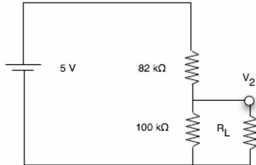
**Figure 3: Voltage Divider.**
