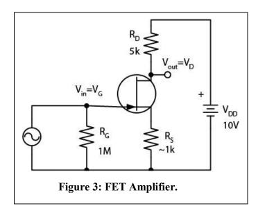
The circuit above is an AC amplifier. The output signal at the drain will be larger than the input signal on the gate.
