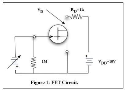
You should find that the drain current decreases with the gate voltage until a point where it is essentially zero. This is the so-called pinch-off voltage. Compare your answer for the pinch-off voltage with the rather liberal limits given on the data page for "Gate-Source Cutoff Voltage".
