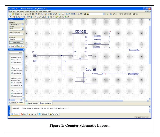
your symbol may be differently ordered than in Fig. 1. Test your design by creating a Testbench Waveform and running the simulation program to see the response of the counter. Be sure to make the clock stream long enough, so that more than 60 output counts are observed. This will ensure that the full functionality of the counter is tested. If your design is successful, create a schematic symbol for your new counter and verify that it is available as a symbol on the schematic entry page.
