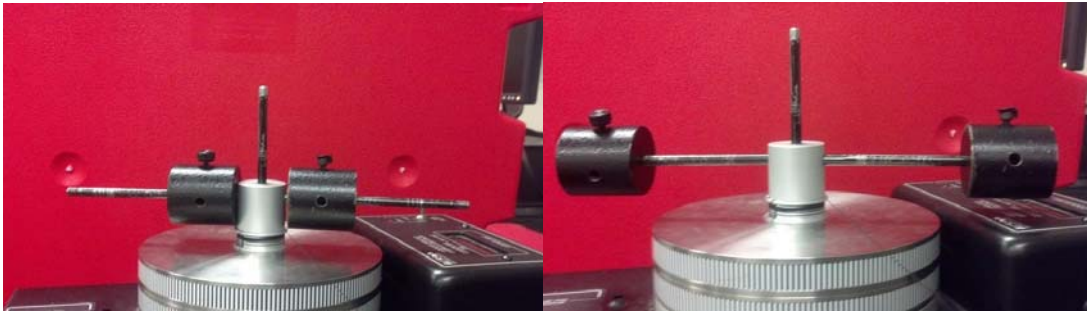
Figure 4: The masses are placed with a small r , all the way in on the left; and masses are placed with a large r , all the way out on the right.
