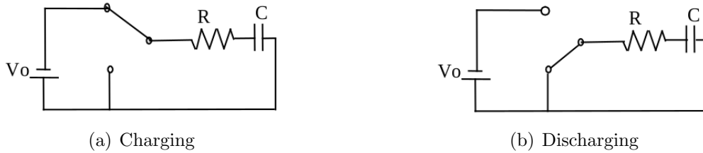
Figure 4.2: Schematics of charging and discharging a capacitor.
