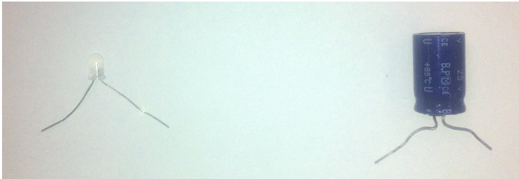
Figure 4.11: The little white object on the left is a light-emitting diode (an “LED”) for the second part of the lab. The blue object on the right is the capacitor that we’ll use in this lab. Both are in the plastic bucket of parts.
