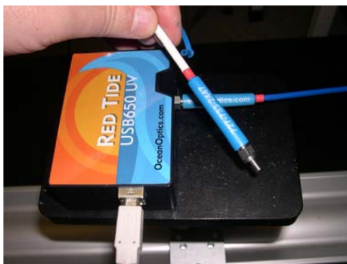
Figure 8.8: The digital spectrometer with a white USB cable and blue optical fiber plugged in.
