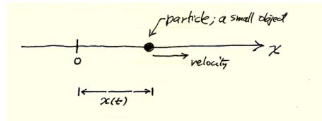
The equations of motion are m dv/dt = F and dx/dt = v.
