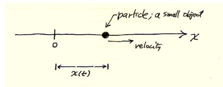
The equations of motion are m dv/dt = F and dx/dt = v.
