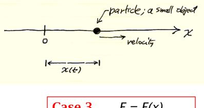
The equations of motion are m dv/dt = Fand dx/dt = v.
