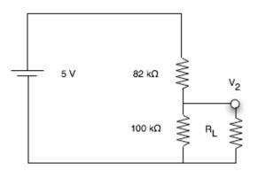
Figure 3: Voltage Divider.
