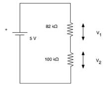
Figure 1: Resistors in Series.
