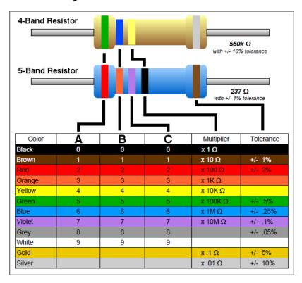
Note: Every time you pick a component, such as a resistor, from a component bin, you should verify whether the value markings on that component agree with your
