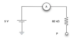
Figure 2: Open Circuit.
