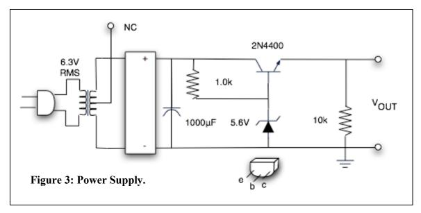
The rectangular box refers to the full-wave rectifier WL02F (alternatively RB152) and "NC" means no connections to the center tap on the transformer. The output should be about 5 volts. *Note*: A commercial full-wave rectifier bridge has 4 terminals, two for AC
