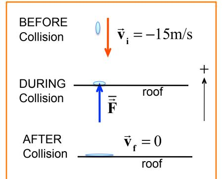
By Newton's 3rd Law average force of raindrops on the roof is
